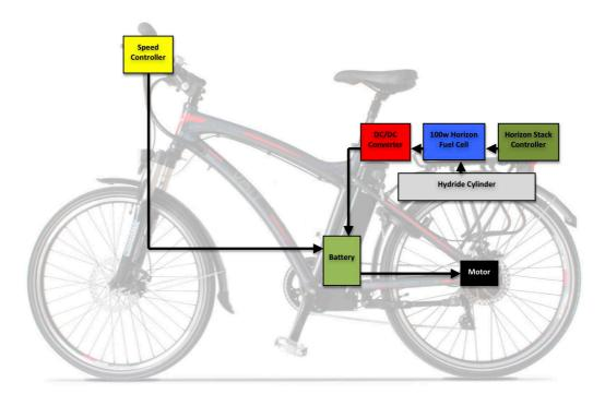
The HMX Electric Bike Kit is a Plug-and-Play hydrogen fuel cell system designed to hybridise with existing electric bikes. The system acts as a range extender, increasing the runtime of any electric bike by providing an additional hydrogen fuel cell energy source.
