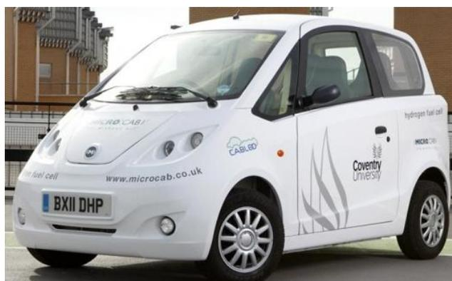
This next-generation hybrid machine brings together expertise from the automotive and motorsport industries, incorporating a chassis designed by Delta Motorsport and Microcab and engineered by Lotus. For the power source of the H2EV, Arcola Energy has installed a system composed of fuel cell, control system and power-conditioning circuitry to charge the vehicle battery while in transit.
