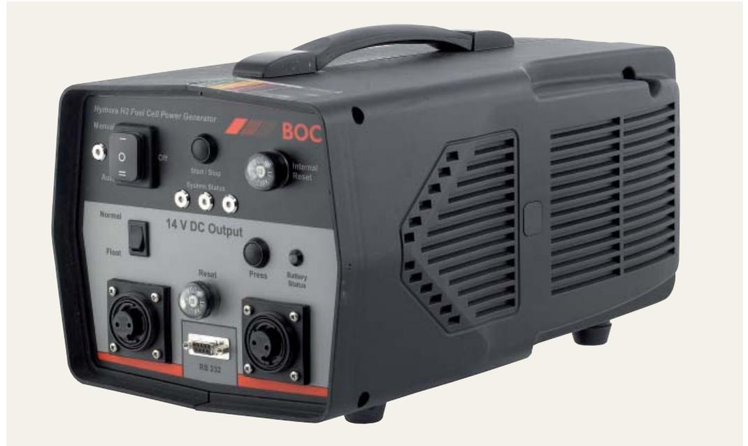
**Description** The Hymera DC is a hydrogen powered fuel cell system capable of delivering 150 W of DC power in off grid and remote locations. This makes it ideal for supplying power for applications such as remote monitoring, control and telemetry stations which can be powered from 12 volt rechargeable batteries.
